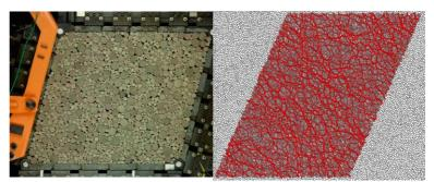
Sheared granular assembly of 2D grains –  $1\gamma 2\epsilon$  device (left). Sheared granular assembly of 2D grains and contact forces – DEM (right)
