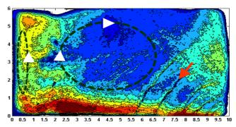
Solute composition map in a Tin-Lead alloy ingot solidified from the lateral sides. Digitalized X-ray image. Dimensions of the ingot 10×6×1cm<sup>3</sup>. The red color corresponds to the positive segregations.
